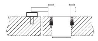
Lock is shown in locked position for right hand door applications.
