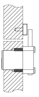
Lock is shown in locked position for standard drawer applications.
