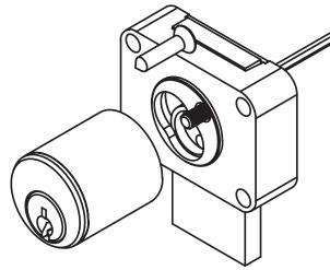
Use a 5/64" Allen wrench from the back to remove the cylinder.
