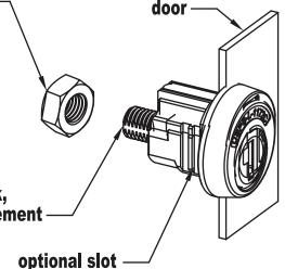
To assemble this lock, use cam from replacement unit here
