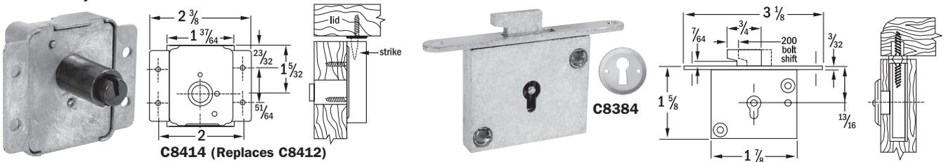
**APPLICATION** – Lid locks for cedar chest application and other lid locking requirements. C8414 is surface mounted and requires a 9/16" diameter hole for cylinder. C8384 requires 11/32" wide x depth of lock full mortise plus mortise for selvedge plus hole for key entry.
