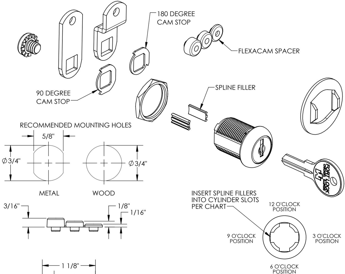
COMBINATIONS OF 2 CAMS AND 3-WAY FLEXACAM SPACER PROVIDE 12 DIFFERENT THICKNESS DIMENSIONS
