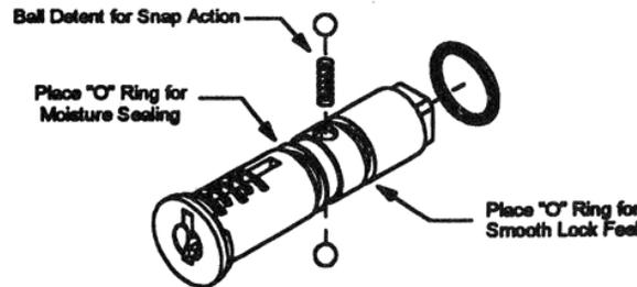
Select the function required and assemble the lock, as specified below
