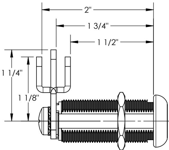
COMBINATIONS OF 2 CAMS AND 3-WAY FLEXACAM SPACER PROVIDE 12 DIFFERENT THICKNESS DIMENSIONS
