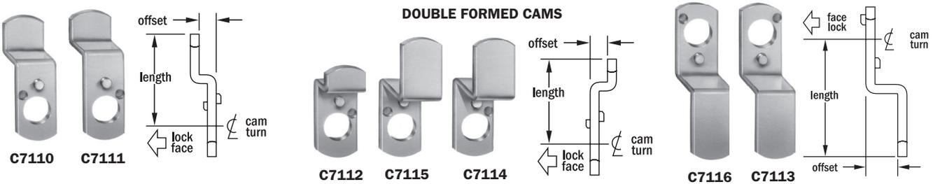
Cams for pin tumbler cylinder cam locks. All cams have dual function. See "Applications" column in table for details.
