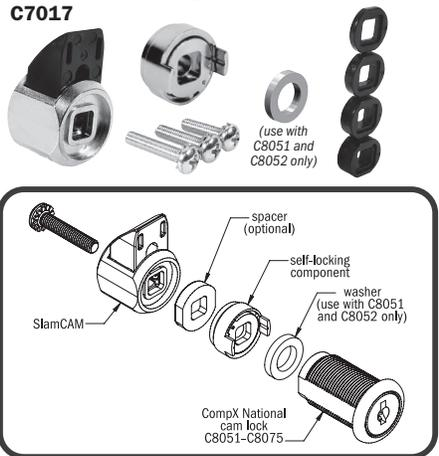
True convenience – release the key, and the self-locking component automatically returns the lock, along with SlamCAM (patent 9,605,455), to the locked position.
