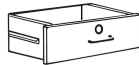
Frame mounted lock - Cam locks on back of drawer front with hook cam engaging strike.
