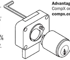
The PLUS feature allows you to remove the cylinder from our pin tumbler box locks while the lock remains in place. No mounting screws need to be removed. Simply use a 5/64" allen wrench from the back to remove the cylinder and plug for re-keying.
