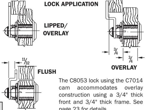
The C8053 lock using the C7014 cam accommodates overlay construction using a 3/4" thick front and 3/4" thick frame. See page 23 for details.
