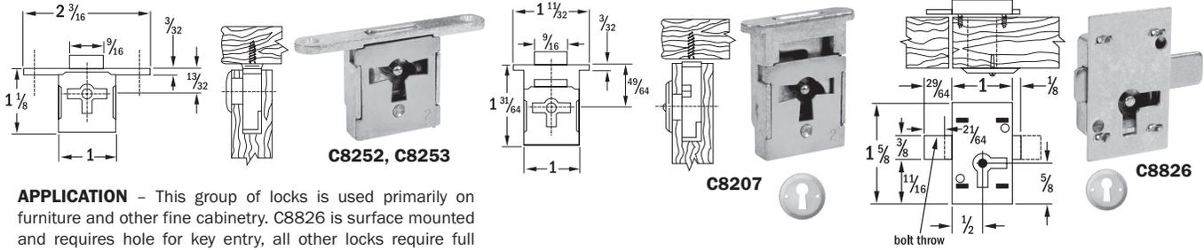
**APPLICATION** – This group of locks is used primarily on furniture and other fine cabinetry. C8826 is surface mounted and requires hole for key entry, all other locks require full 11/32" x depth of lock. Additional mortising, required for lock selvage plus hole for key entry.
