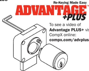
The Advantage Plus feature allows easy removal of the locking cylinder from the lock body without having to remove the lock body from the application. Simply insert a 5/64" Allen tool into the back of the lock and remove the locking cylinder from the front.
