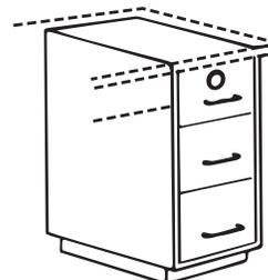
Top drawer mounted lock activates side mechanism securing other drawers.
