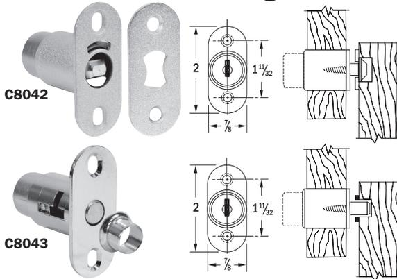
**APPLICATION** - C8040 for glass sliding by-pass doors up to 1/4" thick. C8042 and C8043 for wood sliding doors - requires a 7/8" diameter hole in front door.
