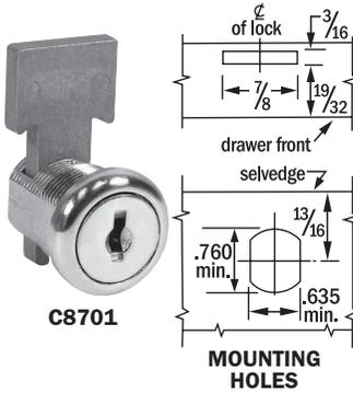
**APPLICATION** - C8701: for center drawers of metal desks. Fits special piercing of drawer front and selvage (see drawing). C8896 is a specific replacement lock.
