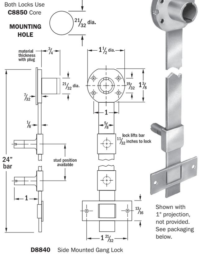
**APPLICATION** – For locking drawers in desk pedestals and other multiple drawer applications. Lock mounts on inside of unit. Surface mounted. Requires 21/32" diameter hole for cylinder.
