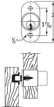
**APPLICATION** - C8140 is for sliding glass doors. C8142 and C8143 are for wood sliding doors and require a 7/8" diameter hole in front door for cylinder. C8150 is used internally on filing cabinets to gang lock drawers.
