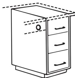
Side mounted gang lock - vertical bar movement - locks all drawers simultaneously.
