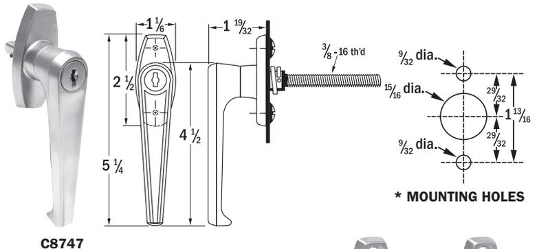
**APPLICATION** - For doors on metal lockers and cabinets. For R.H. doors, install with escutcheon vertical. For L.H. doors, install with escutcheon horizontal. See above drawings. Choice of spindle lengths and mounting. Spindles accept both C8756 latch plate and C8757 tongue except C8747 which has 8-32 tapped end hole and C8749 which will accept only the C8757 tongue. Spindles can be cut to fit special requirements.
