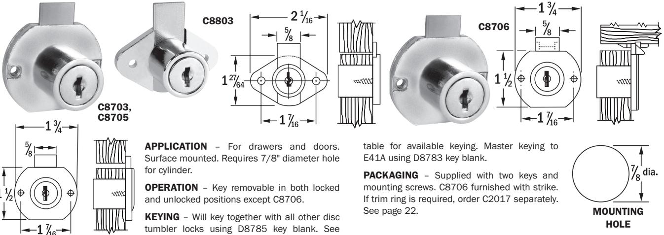
**APPLICATION** - For drawers and doors. Surface mounted. Requires 7/8" diameter hole for cylinder.
