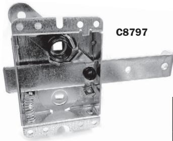
**APPLICATION** – For mounting on sectional over head doors. Factory assembled for R.H. mounting. Mechanism installs at right side of door (inside garage) to lock into track. Handle can replace Overhead Door locking handles. Mechanism can be reversed for L.H. application.
