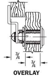
The C8073 lock using the C7014 cam accommodates overlay construction using a 3/4" thick front and 3/4" thick frame. See page 23 for details.
