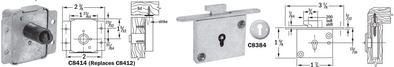
**APPLICATION** – Lid locks for cedar chest application and other lid locking requirements. C8414 is surface mounted and requires a 9/16" diameter hole for cylinder. C8384 requires 11/32" wide x depth of lock full mortise plus mortise for selvage plus hole for key entry.
