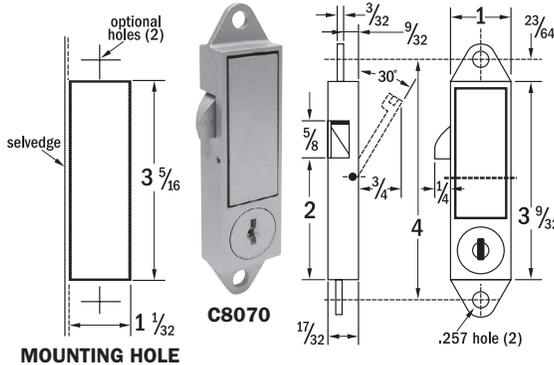
**APPLICATION** – For right handed metal doors of electrical circuit breaker cabinets.
