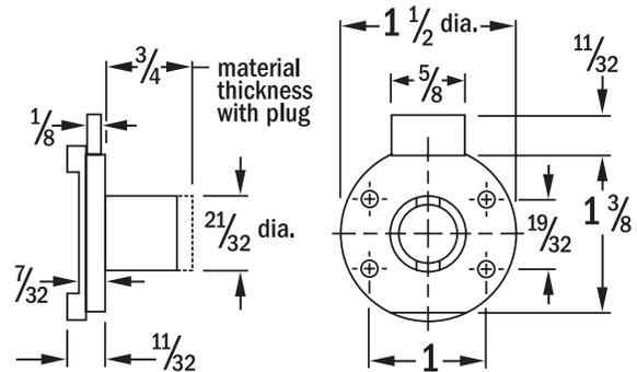
**APPLICATION** - Two drawer "Mini Gang" lock for desk or pedestals, and single locking drawer for desk or pedestals. Surface Mounted.
