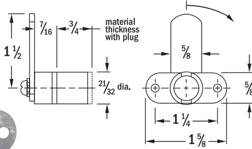
**APPLICATION** - For wood pedestals, door or drawer, R.H. or L.H. Surface Mounted. For flipper door use C7015 offset cam and C2003 strike. See pages 17 and 22.
