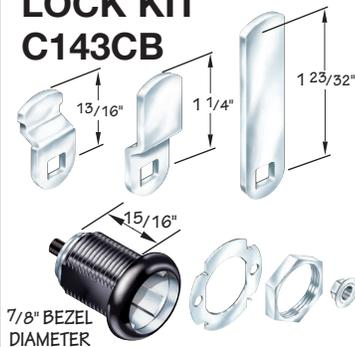
**Application** – Universal type lock for either doors or drawers. Kit will accommodate most locking applications for material thickness 1/16" – 1/2".
